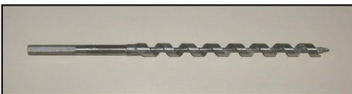
Figure 1: 3/8" Auger Bit
